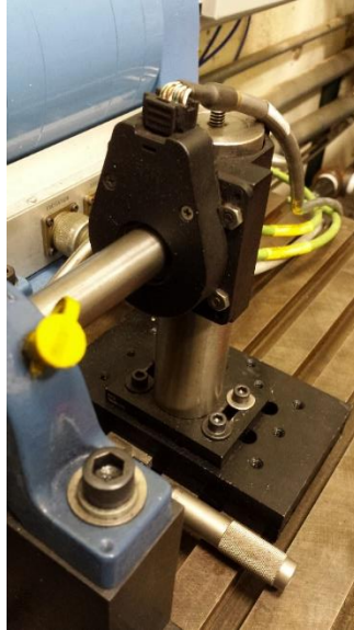
Figure 74. The optical crankshaft encoder from which the encoder pulse and z-pulse originate.
