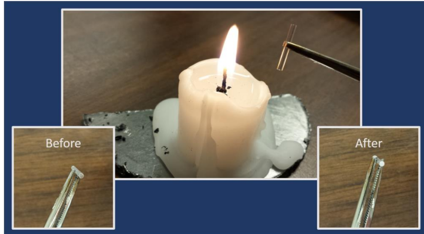
Figure 50. Preparing a sapphire rod for a glue bath by coating optical surfaces with wax.
